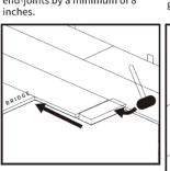
Step 7: Tap end of plank with hammer and tapping block to lock ends of planks together. Remove support bridge and continue with this method until you have completed installing the row. Note: BE SURE TO TAP ON EDGE OF VINYL SO AS NOT TO DAMAGE LOCKING PROFILE.
