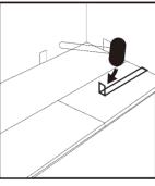
Step 8: Use hammer and pull bar to lock final piece in row. Insert spacer at end of row. Continue installation to final row.
